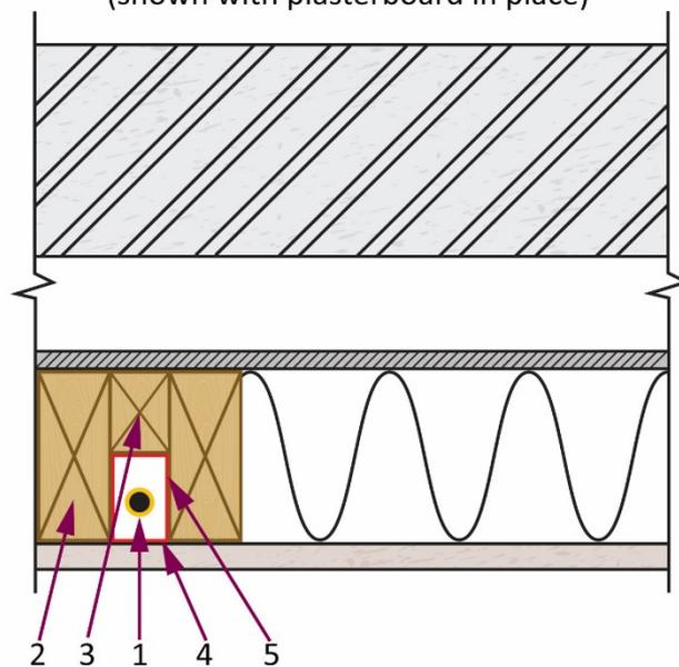
**Note:** Joints between the wall and the studs must be sealed with a suitable mastic to avoid escaping gas tracking around the wooden studs.
