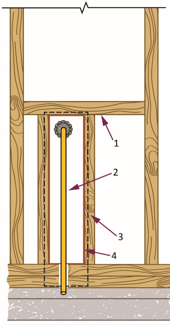
**Note:** Joints between the wall and the studs must be sealed with a suitable mastic to avoid escaping gas tracking around the wooden studs.
