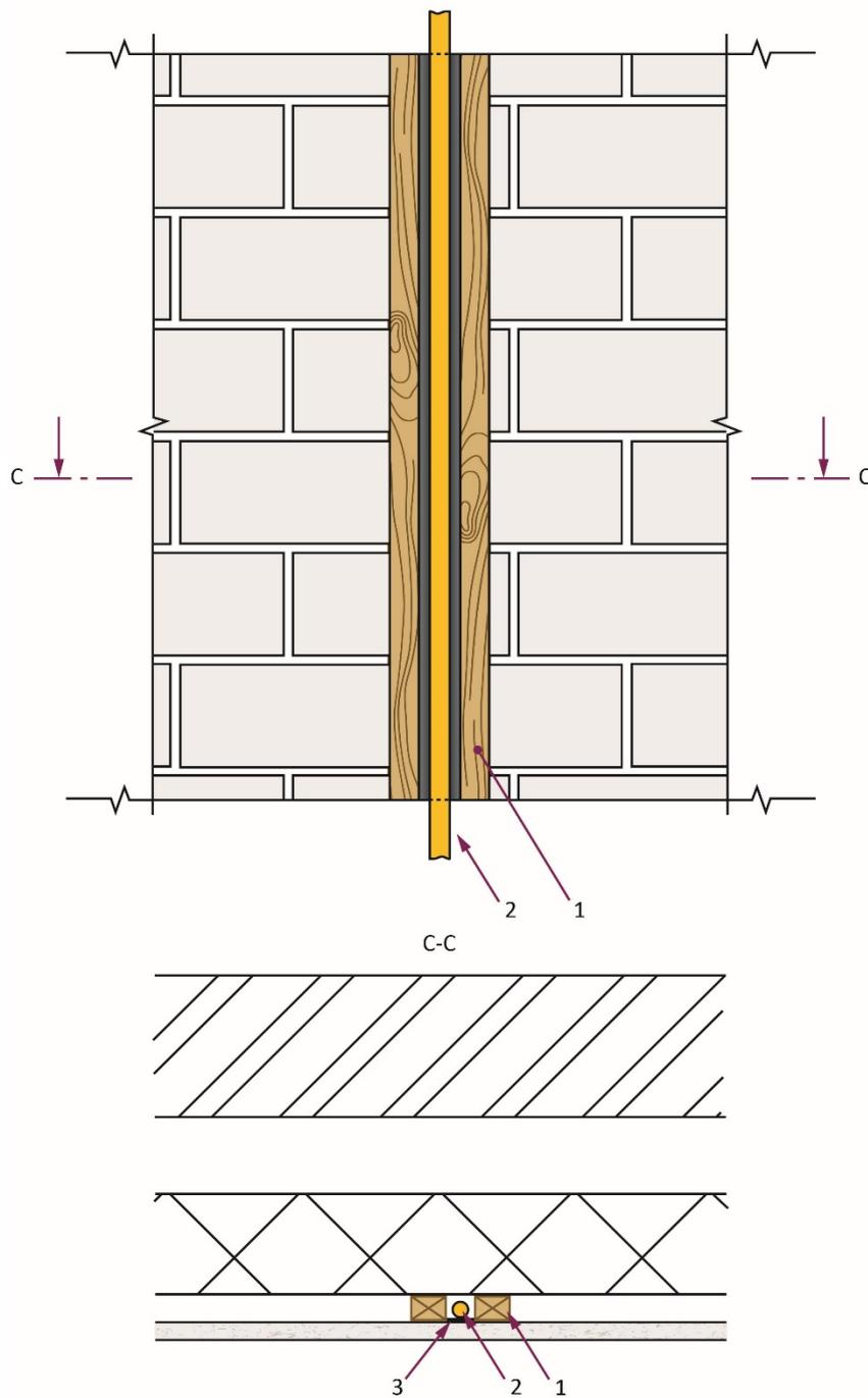
**Note:** Joints between the wall and the studs must be sealed with a suitable mastic to avoid escaping gas tracking around the wooden studs.
